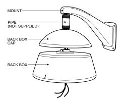
Figure 1. Back Box Cap and Back Box Installation
